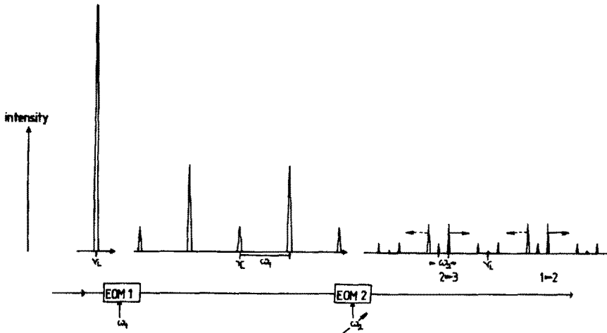
Fig. 2: Schematic frequency spectrum of the cooling laser beam behind the two electro-optic modulators (EOM). The cooling and repumping sidebands are marked 2=3 and 1=2.
